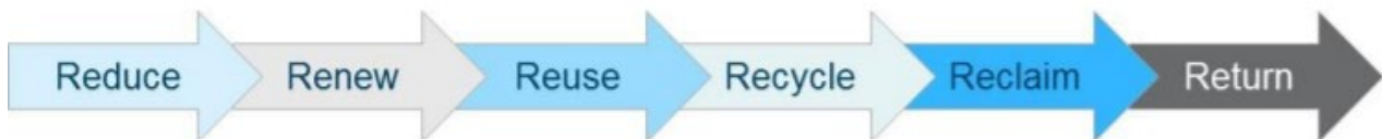
Figure C.5: 6R approach - Prioritized route to reduced and more efficient industrial water use. Reduce: through (simple) better in-house water management schemes; Renew: introducing more water efficient technologies; Reuse/Recycle: Direct reuse in other processes with lower water quality demands or recycle in the same process; Reclaim: Treatment of process stream to required quality and reuse/recycle in the same or other processes; Return: Discharging remaining wastewater to own or municipal wastewater treatment plant.
